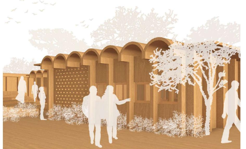
Jack arch vault roofs for column free long span spaces, the curved surface reduces heat gain
