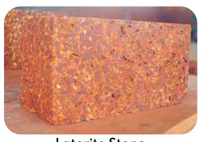
Laterite Stone Commonly used in foundations, most vernacular houses are constructed in load bearing techniques with isolated footing
