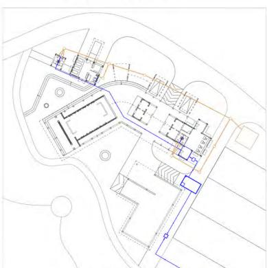
Fig. 67. Water Supply and Drainage Layout
