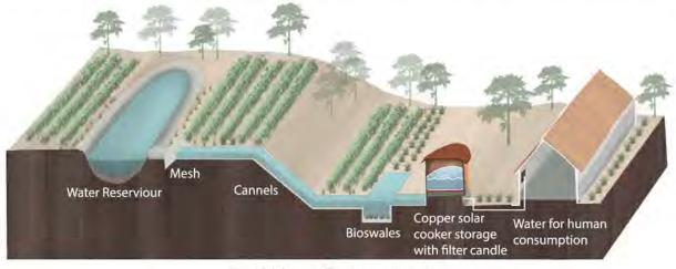
Fig. 80. Water purification supply system
